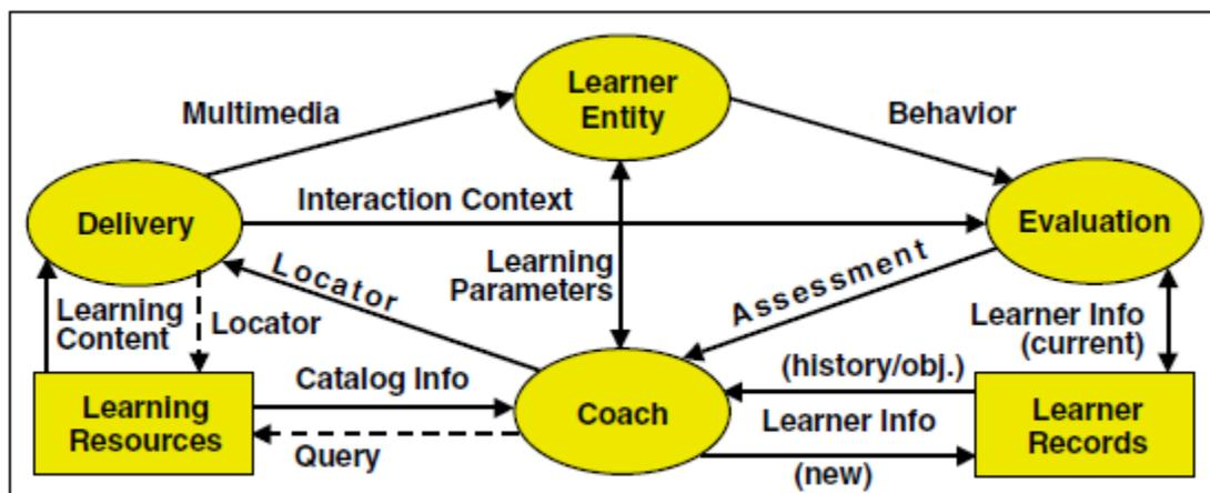
Figure 1: The LTSA System Components
